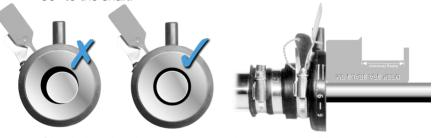
**5.** Check that the shaft is central to the sterntube, this ensures that the engine is correctly aligned and that the seal will run concentric to the shaft.
